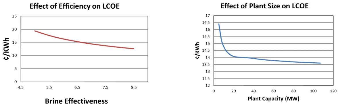
**Figure 5 Sensitivity of LCOE to plant efficiency and capacity at Mountaineer, WV**
